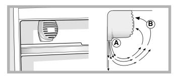
The Aircooler maintains a constant fridge temperature to keep food fresher for longer and will quickly restore the temperature to the correct level, even if the door is opened frequently: the blown air (A) is cooled when it comes into contact with the cold wall, whereas the hotter air (B) is sucked up (see diagram).
